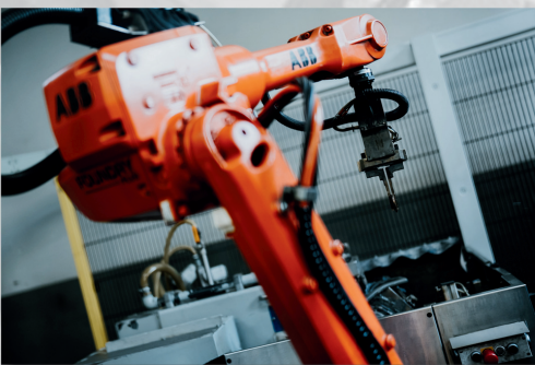
Robotic grinding process for straw choppers
