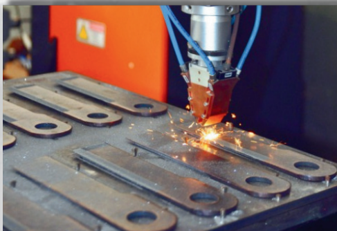
Laser deposition of hardened carbide layers
